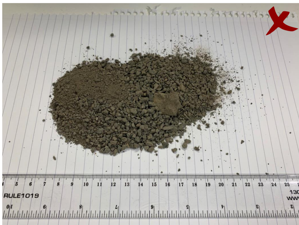
Figure 30 - Examples of non-compliant bedding material – Gravel
