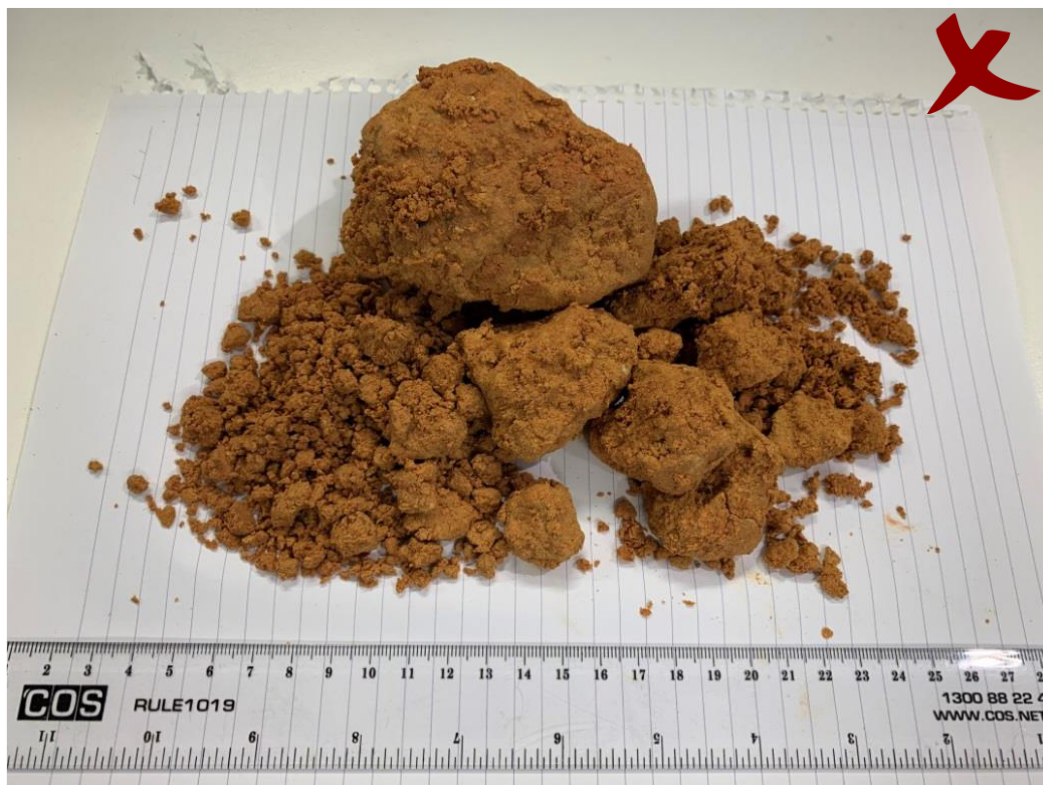
Figure 29 - Examples of non-compliant bedding material - Sand containing clay
