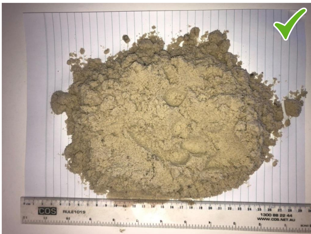
Figure 28 - Examples of compliant sand
